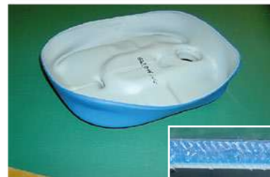
Test with nitric acid to check the chemical compatibility
