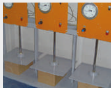
Stacking test 3m x 24h
