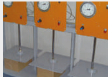
Stacking test 3m x 24h (calculated according to the weight and height of the box x 24h)
