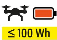
For this type of battery, when packed with the device ("packed with"), **the package is required to pass a 1.2 m drop test**. These tests must be documented and filed.
